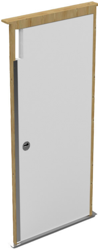
HOISTWAY VIEW WITH 1/8" SHEET-METAL STOPPER
